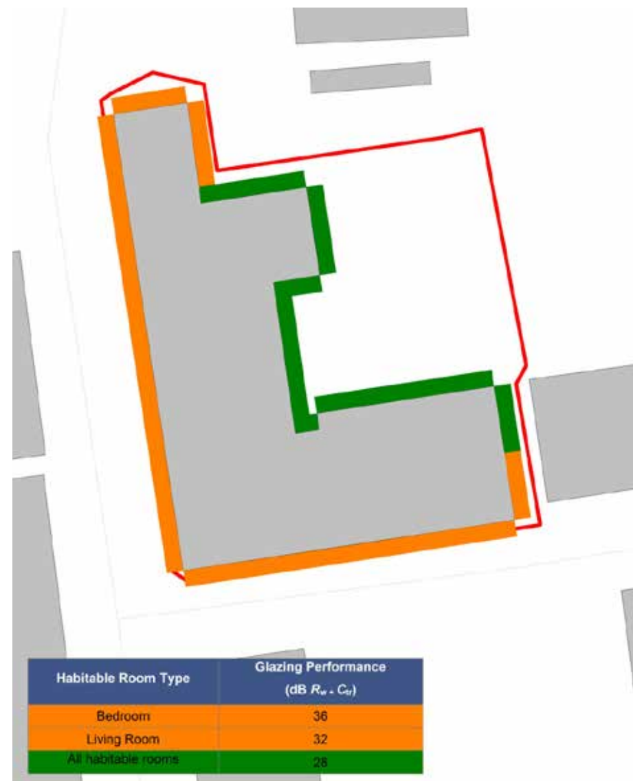
Fig 13 - Proposed Facade sound insulation area and glazing performance
